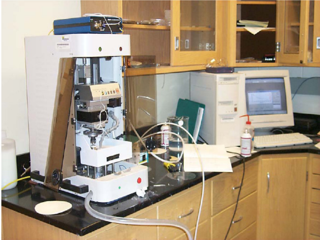
Figure 3.6 Universal Micro Tribometer with PC Based Feed Back Control
